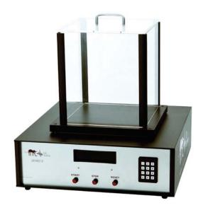
The IITC Hot Plate Analgesia test is used for latency testing in rats and mice. The animals are placed on a black anodized, aluminum plate (11" X 10.5" X ¾", 275mm X 263mm X 15mm) which is heated uniformly.
