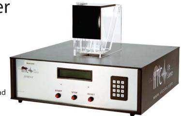
The IITC Incapacitance Test Meter is used for test assessment of pain and or inflammation of the hind limbs on mice, rats and birds. It overcomes the drawbacks of other methods that might cause unnececessary stress or subjectivity on the animal. The technique known as dynamic weight bearing enables the test on both limbs allowing a clean stress free correlation to the paw pressure test. Control and testing can be done on the same animal at the same time.
