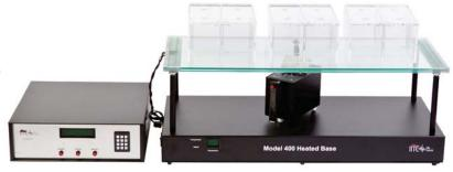
Three individual, acrylic animal enclosures are supplied. Each enclosure allows for 2 rats/4 mice allowing testing of up to 6 rats/12mice total. Enclosures have strong magnets to prevent animals from possible escape with individual lids and clear dividers in-between test subjects for easy viewing.
