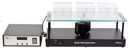
The IITC Plantar Analgesia Meter for thermal paw can be used on 12 mice, 6 rats and other animals (cats, rabbits) unrestrained when testing for narcotic drugs. Experiments are easy to perform, simply slide the test head under test subject, align the heat source via our exclusive guide light (idle state) by the attached, adjustable, angled mirror on test head to test subject and perform tests.
