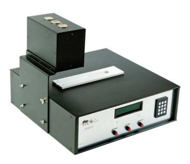
The IITC Tail Flick Test apparatus meter measures latency and/or temperature threshold when detecting properties of narcotic and strong non-narcotic drugs on mice and rats. A built-in Timer is automatically stopped when the animals' tail flicks out of the beam of light, test result will be displayed on readout for viewing.
