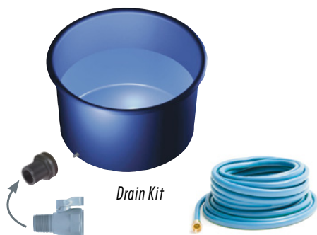
Bulkhead fitting (pre-mounted on tank) provides drain hole with 3/4" FIPT to connect Drain Kit or user supplied drain piping
